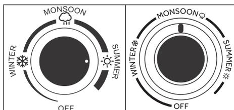
Temperature inside refrigerator can be set by control knob.
